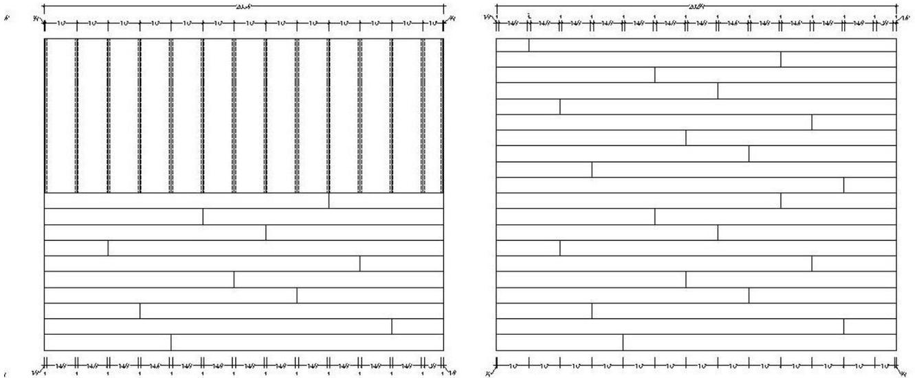
**END-TO-END SEAMS/JOINTS OF 'QUICK-LOCK' PLANKS
