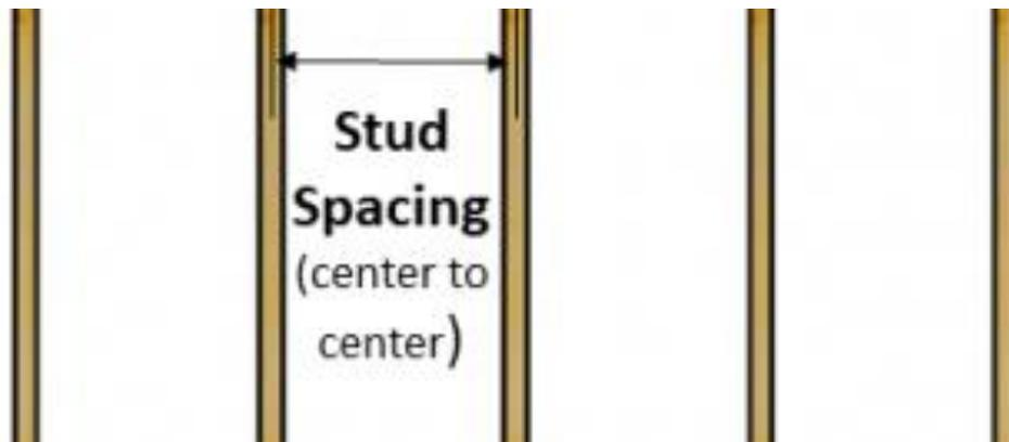
Once you have identified the on-center joist or stud spacing, your T&G Planks will need to be fastened at each of the joist and/or stud locations.
